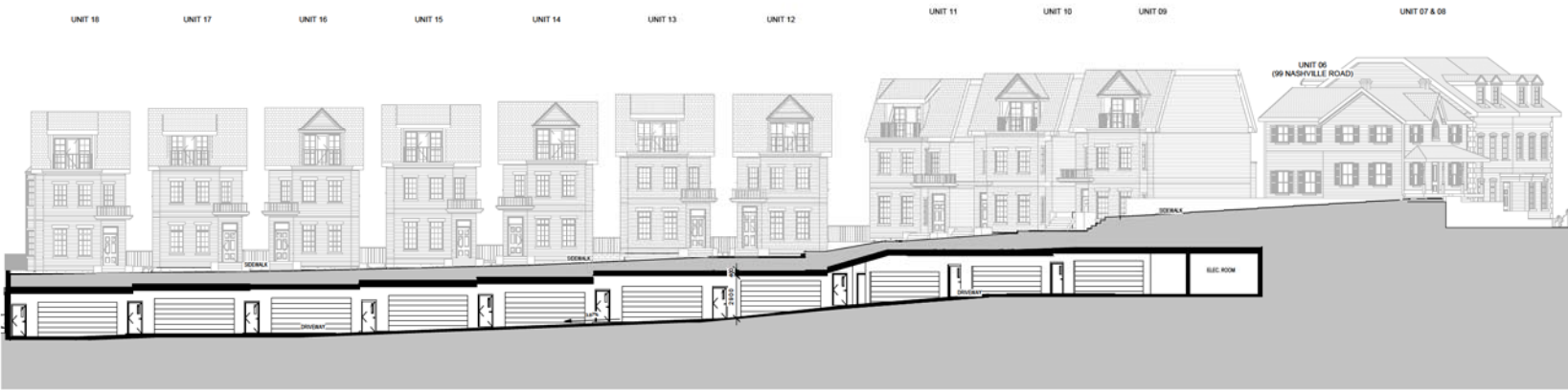
2 WEST SITE SECTION AS-02 1:150 0m 3m 6m 9m 12m 15m VISUAL SCALE 1:150
