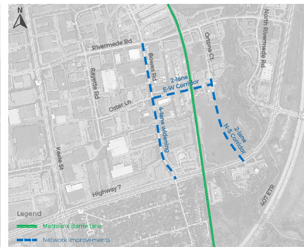
Scenario 4: Scenario 3 + four-lane widening of Bowes Road (between Rivermede Road and Highway 7)
