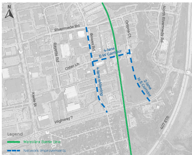
Scenario 5: Scenario 4 + a new four-lane east-west corridor connecting Bowes Road and Ortona Court
