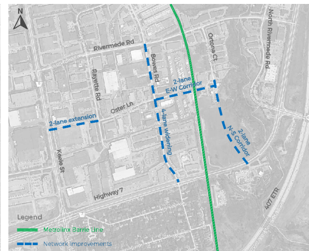
Scenario 7: Scenario 6 + a new two-lane east-west corridor extending Keele Street and north-south corridor (including an existing segment of Oster Lane)
